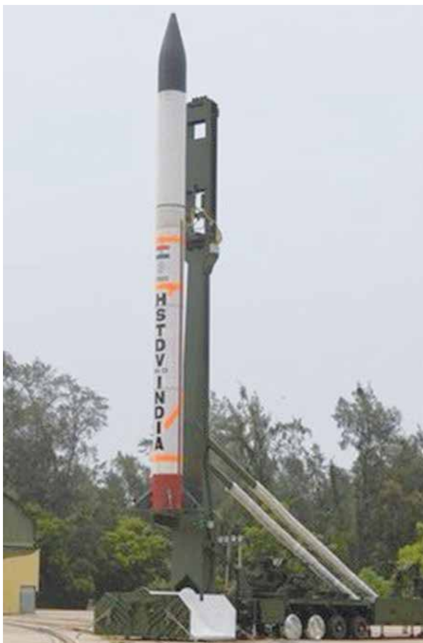
Hypersonic air-breathing scramjet technology with the flight test of Hypersonic Technology Demonstration Vehicle (HSTDV).
