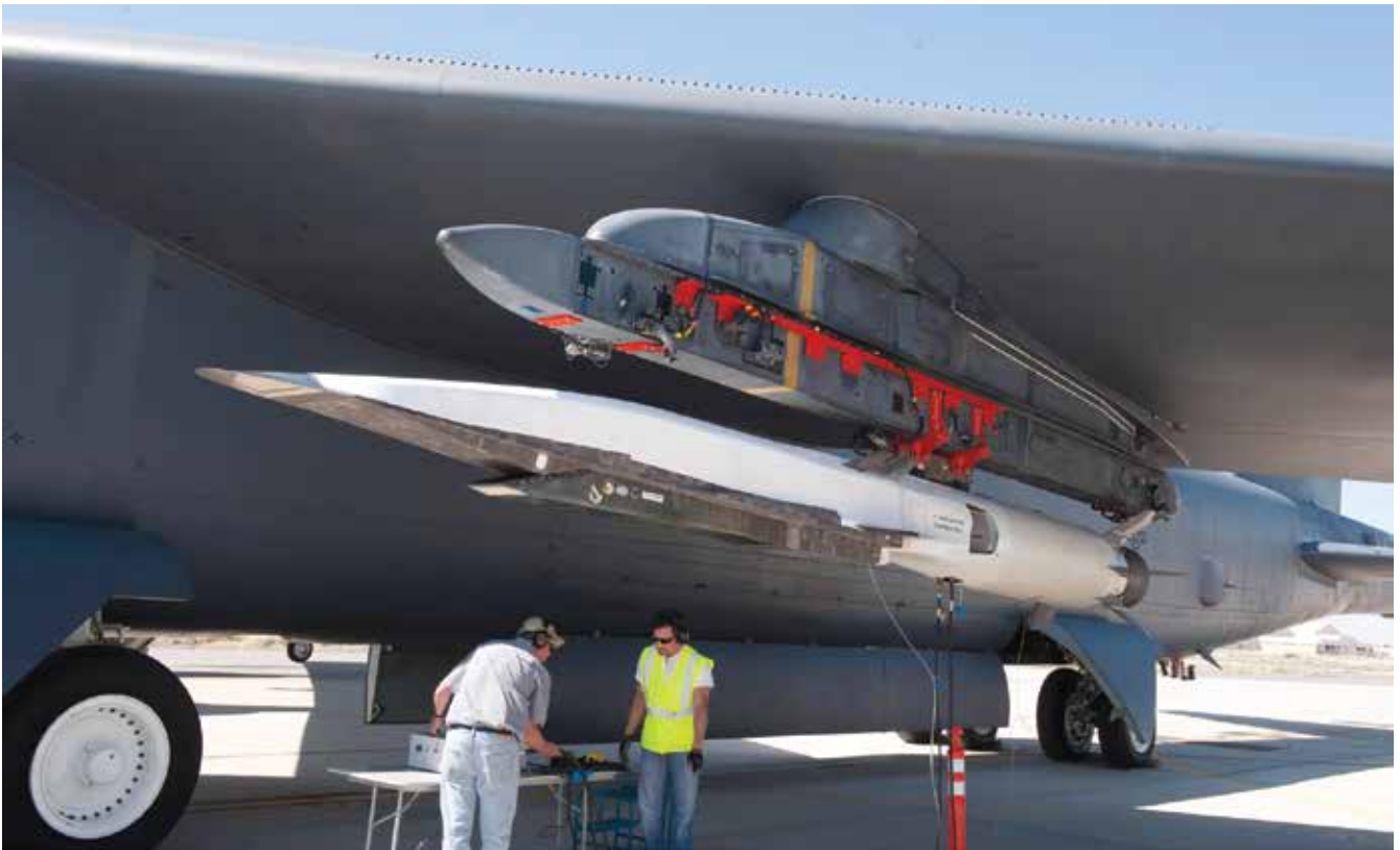
The X-51A Waverider scramjet, which is affixed to an Edwards B-52H Stratofortress.
