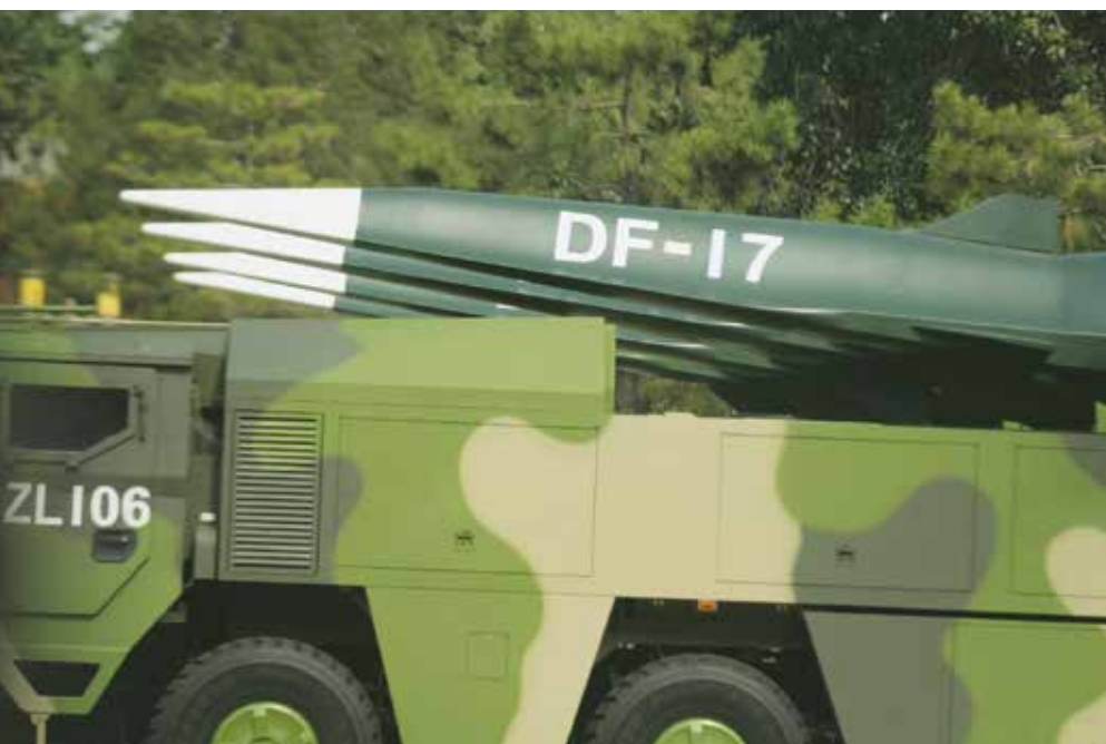
China's DF-17 missile has a hypersonic glide vehicle that can deliver both nuclear and conventional payloads.
