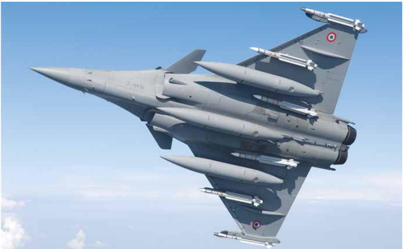
*RAFALE-M Armed with 2-MICA-IR Short Range & 4-MICA-RF Medium Range Air to Air Missiles.*
