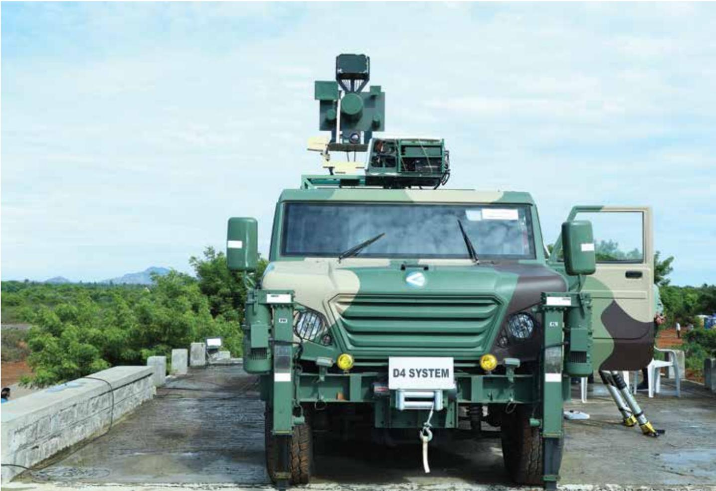
India's Naval Anti-Drone System made by BEL and developed by DRDO.
